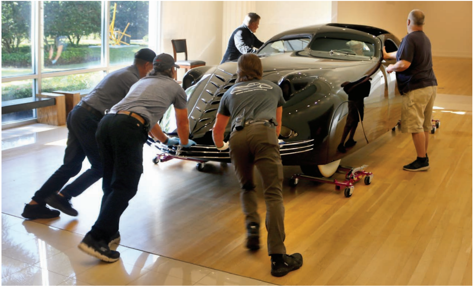
Being careful not to apply pressure directly on the aluminum body, trained staff roll the Phantom Corsair through the museum to its display space.
