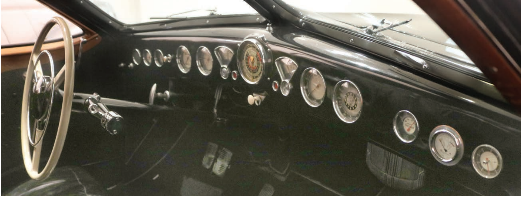
An array of 13 gauges includes a complicated dial in the center that displays pulling power, tractive and wind resistance, brake power efficiency, and more.
