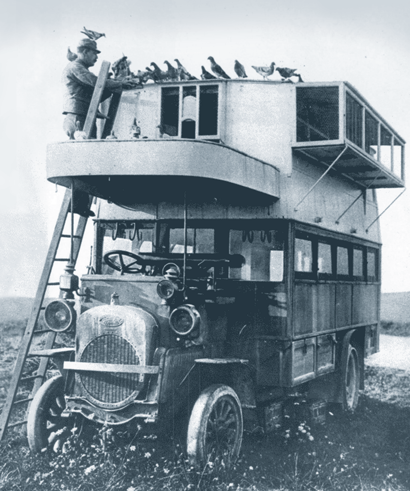
Mobile lofts, such as this converted bus, were used during World War I.
